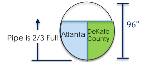
Dry Weather Flow in Peachtree Trunk
